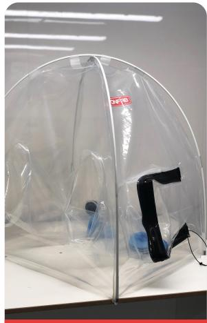
The pop-up isolator can be set up in less than 2 minutes
